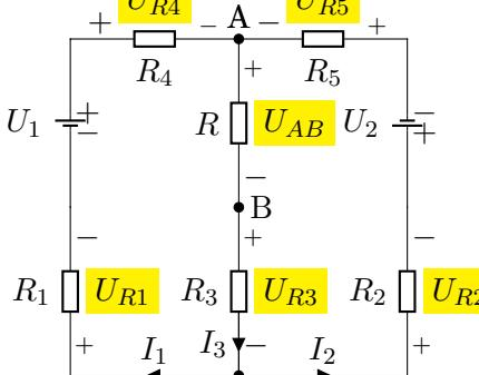
$$\begin{array}{ll} I_3 = I_1 + I_2 & (1) \\ U_{R1} - U_1 + U_{R4} + U_{AB} + U_{R3} = 0 & (2) \\ U_{R2} + U_2 + U_{R5} + U_{AB} + U_{R3} = 0 & (3) \end{array}$$
