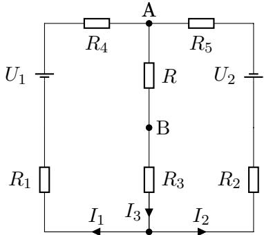
$$\begin{array}{ll} U_1 = 31 \text{ V} & R_3 = 4 \Omega \\ U_2 = 4 \text{ V} & R_4 = 7 \Omega \\ R_1 = 3 \Omega & R_5 = 14 \Omega \\ R_2 = 6 \Omega & U_{AB} = 6 \text{ V} \end{array}$$
